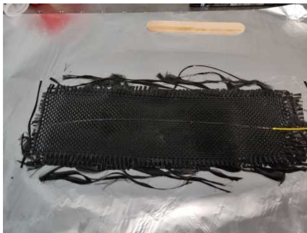
Figure 9: Embedding of optical fiber in carbon plate.
