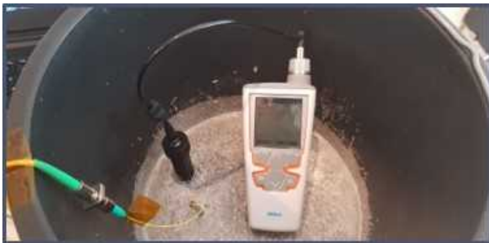
Figure 7: Image of the dry concrete with the Vaisala HM40 probe and the SHUTE sensor inserted into the concrete.
